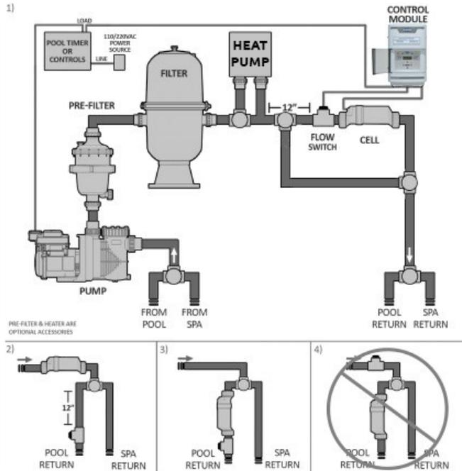
The chlorinator's cell must be installed on the return circuit downstream from the filter and any heating systems (particularly electric heater)
