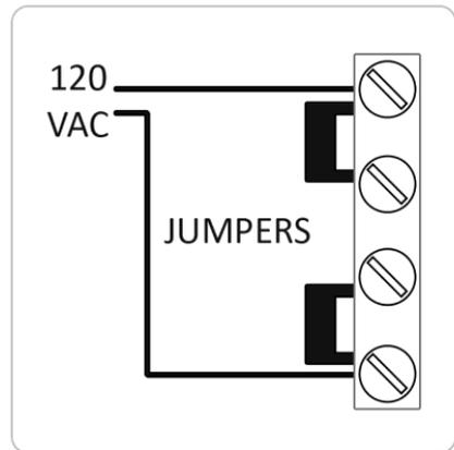
This set of terminal screws can be located inside of the Control Module, and accessed by removing the six screws from the Control Module's aluminum base. The factory voltage setting is the 240V configuration, with a jumper clip inserted between the second and third terminals. The Control Module can be made to accept 110V by reconfiguring the jumper clips as shown above left, with two jumper clips instead connecting the first and second terminals, and the third and fourth terminals.
